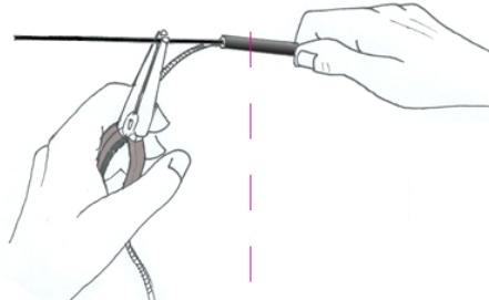
7. When the cord has been threaded through all of the poles, detach and withdraw the wire then place a washer onto the shock cord. Stretch the cord app. 16cm out of the pole and tie a knot to retain the washer.
